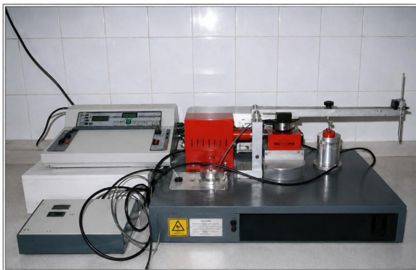
Figure 1. TE91 pin-on-disc tribometer used for the dry sliding wear tests.
