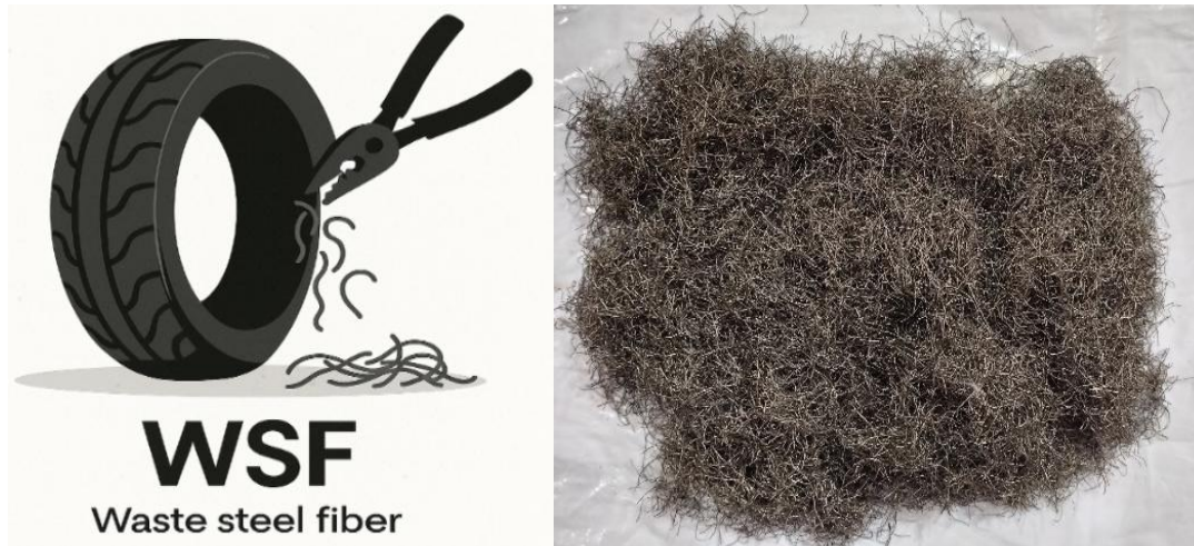
Figure 1: WSF extracted from discarded tires and prepared for use in SMA mixtures.
