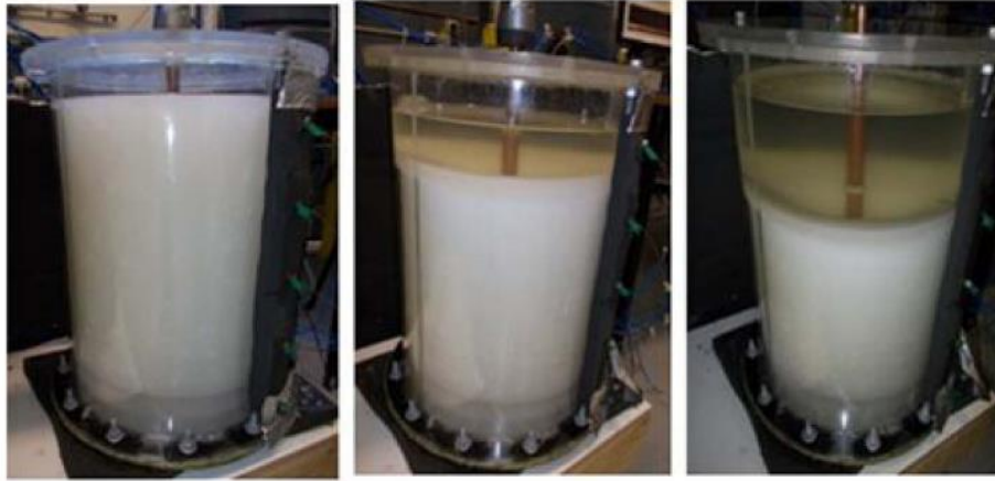
Figure 10. PCM melting in tabular thermal storage unit (Saeid et al. [16]).
