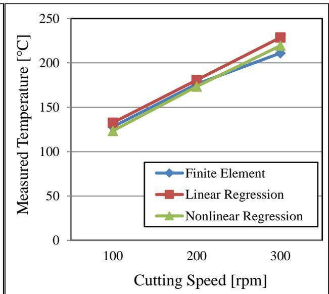
**Figure 14** The variation of temperature vs. cutting speed for feed of 0.15 mm/rev, tool 118°.
