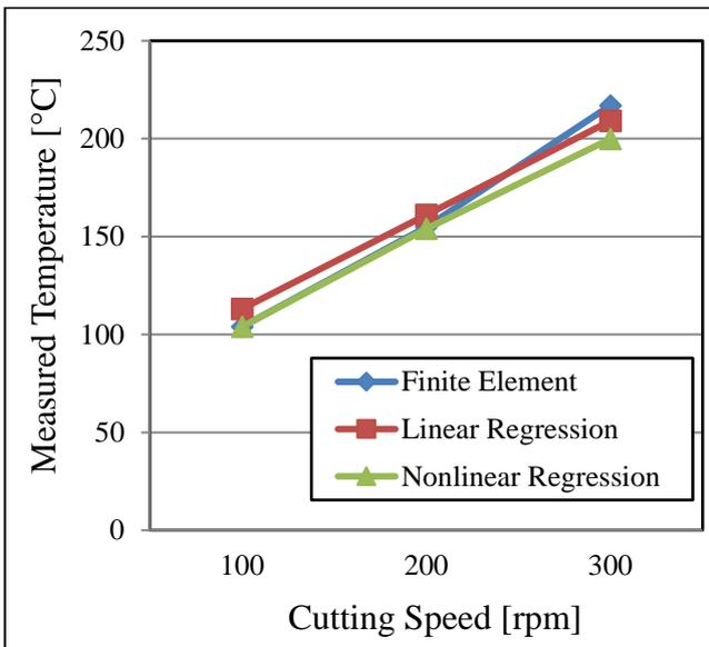
**Figure 13** The variation of temperature vs. cutting speed for feed of 0.35 mm/rev, tool 110°.
