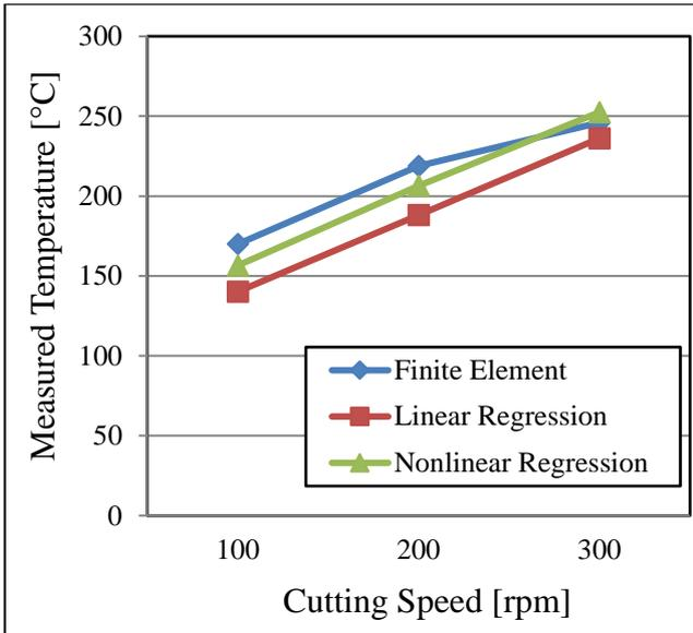
**Figure 15** The variation of temperature vs. cutting speed for feed of 0.25 mm/rev, tool 118°.
