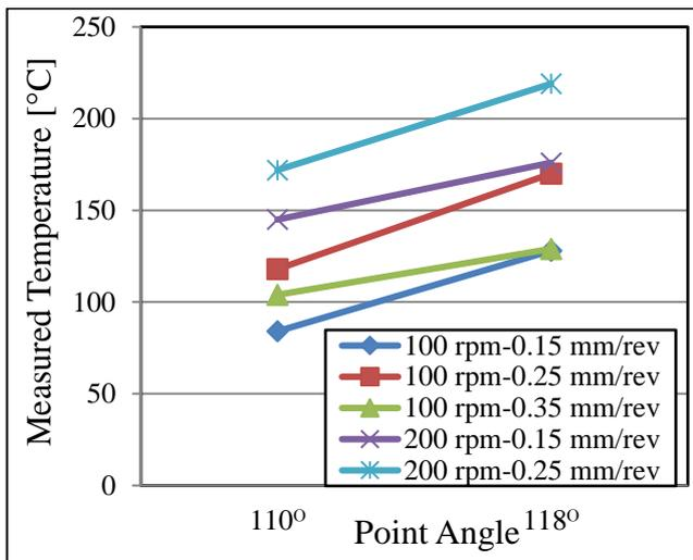
**Figure 9 The variation of temperature with respect to point angle for five FE operations.**
