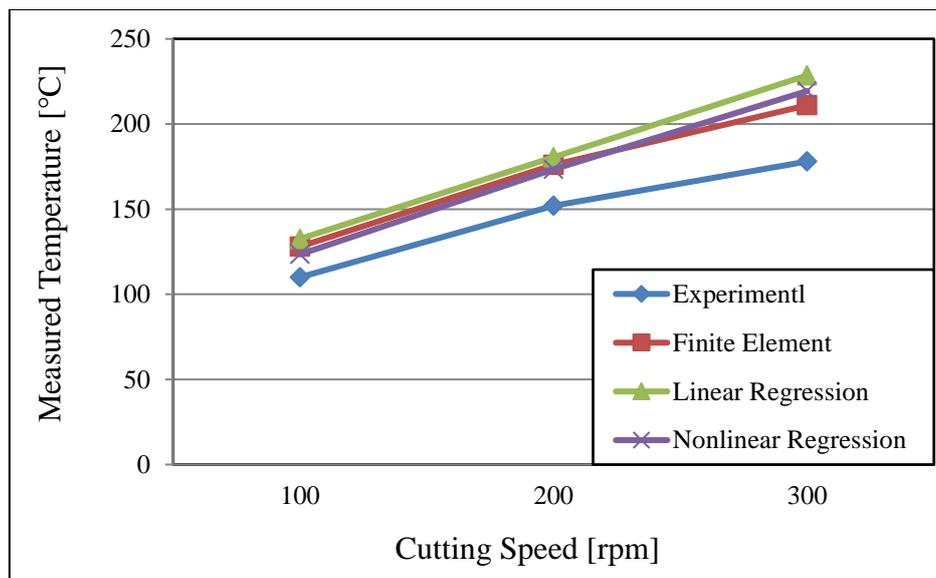
**Figure 17** Variation of temperature vs. cutting speed for experimental, its FE validation and SPSS.
