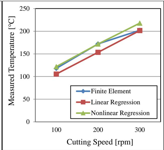
**Figure 12** The variation of temperature vs. cutting speed for feed of 0.25 mm/rev, tool 110°.
