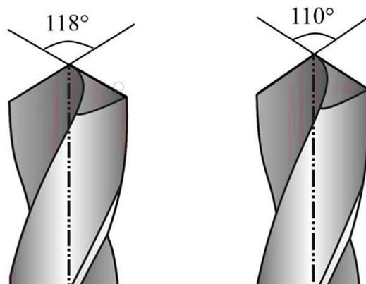
**Figure 2 The point angles of both cutting tools.**
