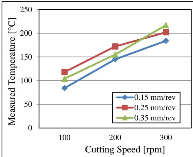
**Figure 5 The variation of temperature with respect to cutting speed at tool of 110° point angle.**
