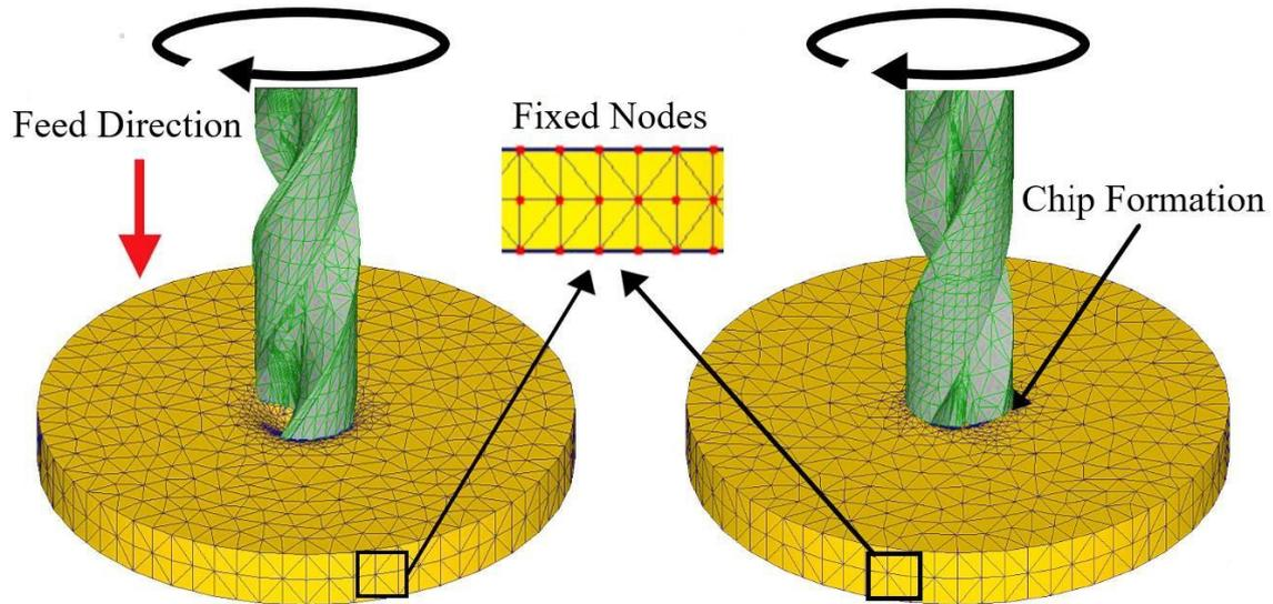
**Figure 3 Constraints of the workpiece model showing the mesh model of tool and workpiece.**
