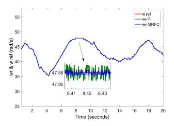
Fig.10: Tracking response of rotor with reference speeds for PL and MREC
