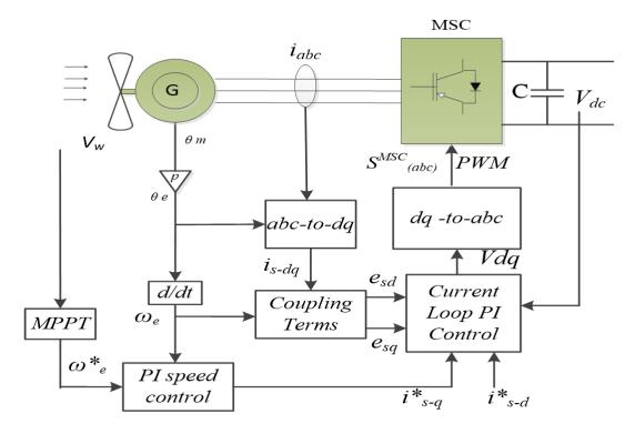
Fig. 4: The schematic diagram of the machine side PI control
