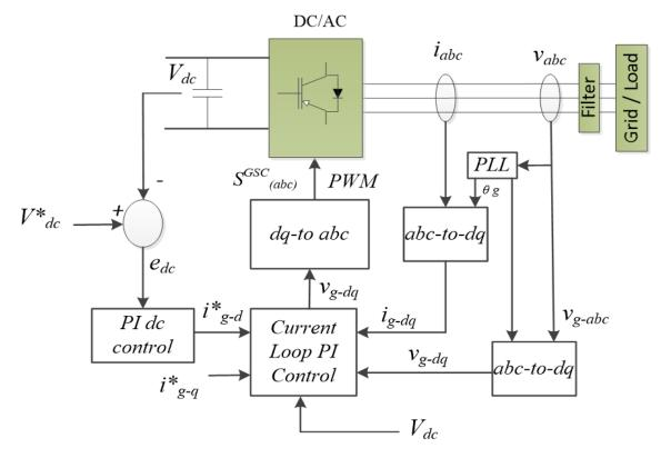
Fig. 5: The schematic diagram of the grid side PI control
