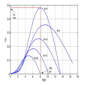
Fig. 2: Graph of power coefficient against TSR
