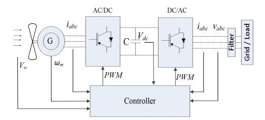
Fig. 1: Wind Energy Conversion System Diagram
